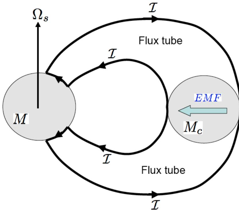
$$\text{EMF : } \Phi = \frac{2\mu R_c}{ca^2} (\Omega_{\text{orb}} - \Omega_s)$$
