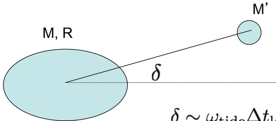
$$\delta \sim \omega_{\text{tide}} \Delta t_{\text{lag}} \sim 1/Q$$
