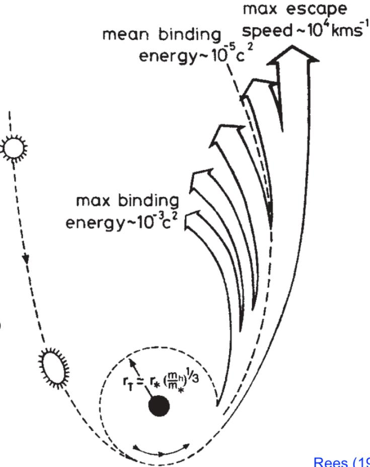
Disrupted stellar debris falls back onto an accretion disk
