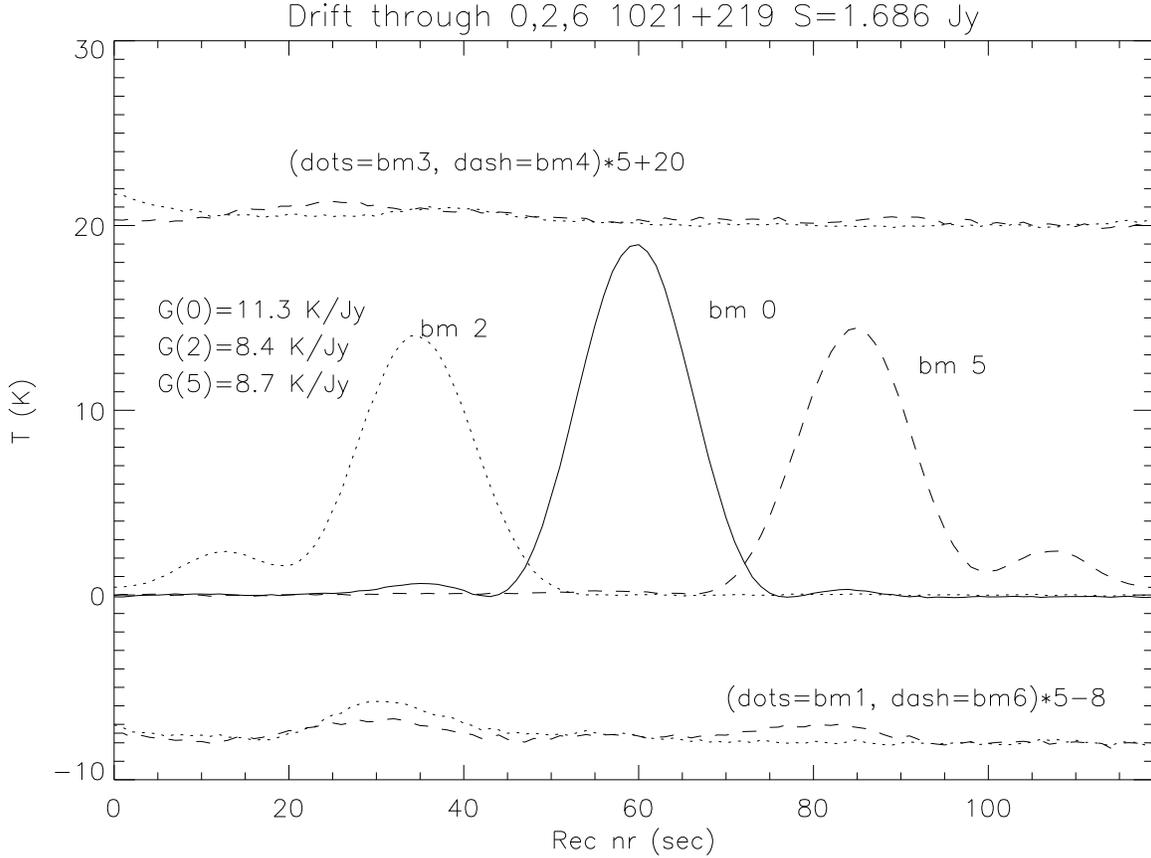
Fig. 1.— Drift 1: continuum power with source 1021+219 going through beams 2, 0 and 5. Tracings for the N group (beams 3 and 4) and from the S group (beams 1 and 6) were blown up by a factor 5 and offset for overplotting.
